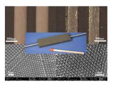
Low temperature catalytic combustion of propane over Pt-based catalyst with inverse opal microstructure in a microchannel reactor
